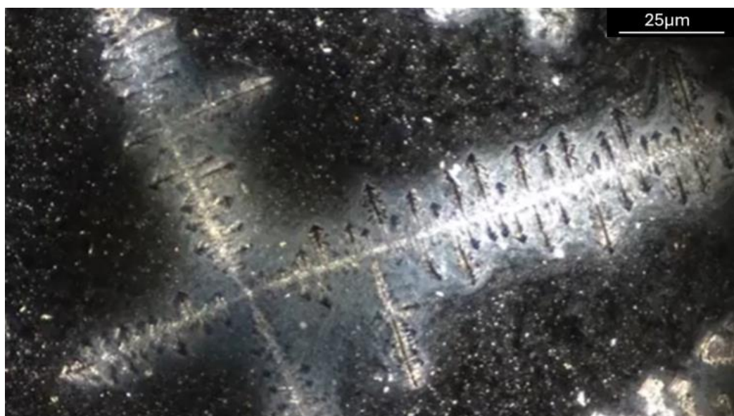
Figure 29. Needle-like crystals formed during Sessile Droplet Evaporation (SDE) with the addition of more sample during the liquid phase. The distinctive black tips highlight a unique crystallization feature resulting from this manipulation. Magnification 100x.
