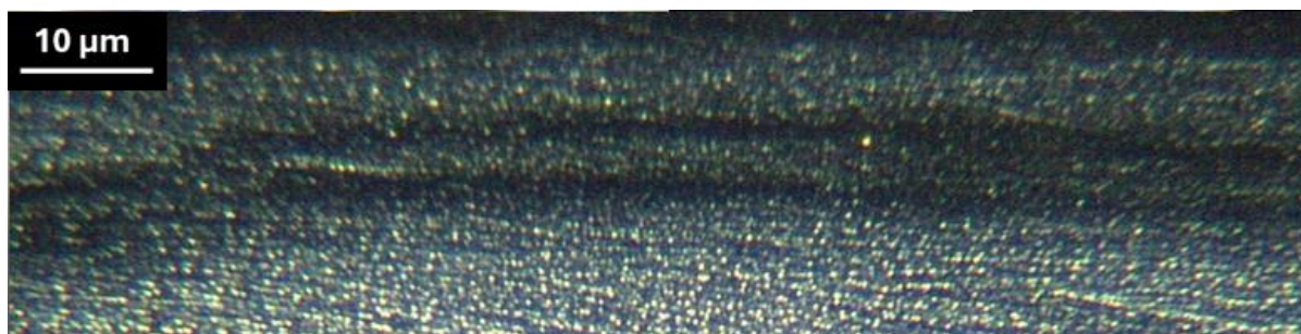
Figure 127. RO water showing minimal particulate matter. Magnification 100x.
