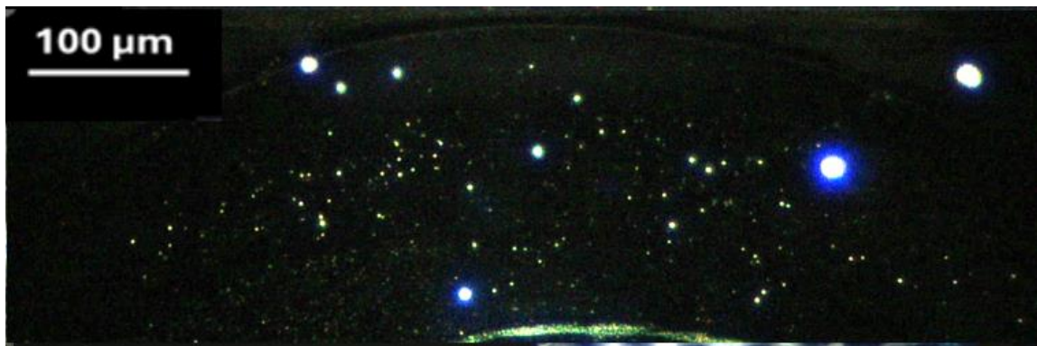
Figure 140. Drop of tap water showing dispersed colloids and larger reflective contaminants under dark field microscopy. The bright points indicate suspended particles, while the larger reflections suggest mineral or environmental impurities typical of hard water. Magnification 25x.
