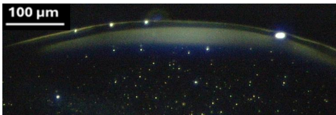
Figure 137. Rosewater with numerous small particulates. Magnification 25x.
