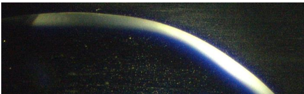
Figure 147. Initial drying pattern of PEG 400 solution, showing a curved drying edge with dispersed particulates throughout the field, indicative of the solution's hygroscopic properties. Magnification 25x.
