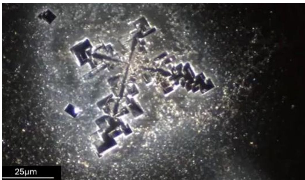
Figure 31. Complex geometric crystal formations resulting from SDE manipulation. The structures exhibit hierarchical assembly and precise modular organization, showcasing the impact of environmental gradients and solute dynamics on self-assembly processes. Magnification 100x.
