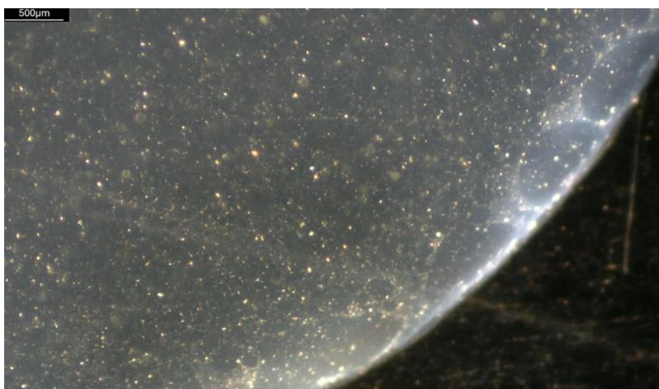
Figure 2. Sessile droplet shortly after evaporation begins, showing a smooth circular boundary driven by capillary flow. Reflective particles distributed throughout the droplet indicate high-density colloidal material initiating crystallization and early self-assembly. Magnification 25x.
