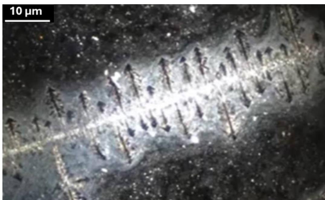
Figure 30. Close-up view of the needle-like crystals, emphasizing the black tips at the branching termini. This detail reveals localized solute dynamics and material variations within the manipulated crystallization environment. Magnification 200x.
