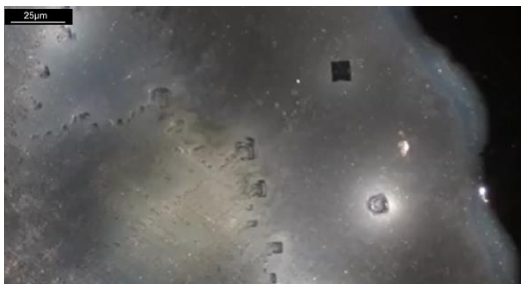
Figure 36. A broader view near the droplet edge showing distinct crystal formations influenced by colloidal distribution in this region. This image highlights the relationship between environmental gradients and the variability of self-assembly outcomes. Magnification 100x.
