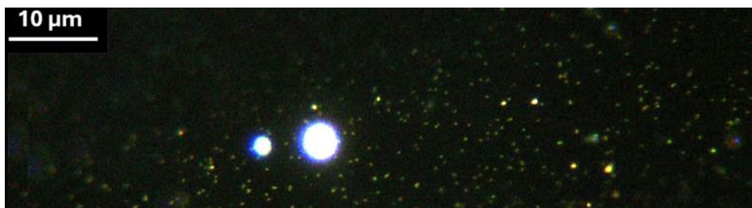
Figure 141 showing dispersed colloids and larger reflective contaminants. The colloids appear as fine, bright points, while the larger, intense reflections indicate mineral or particulate impurities. Magnification 100x.
